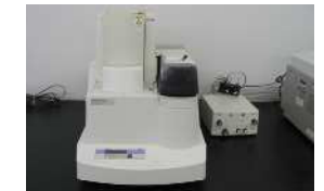
⑦熱重量-示差熱同時測定装置 TG-DTA Thermogravimeter-Differential thermal analyzer 物質の熱分解温度、分解量の定量、付着水や結晶水の定量、脱水温度等を測定します。 Measures decomposition temperature, quantitative determination of decomposition, adhering water, crystal water and dehydration temperature etc.
