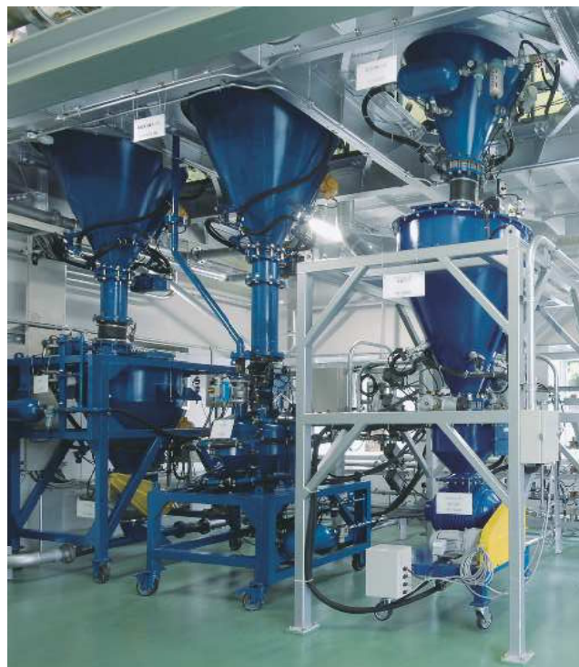
③多目的ライン(1) Granular/Powder conveyance test line for general use (1)
