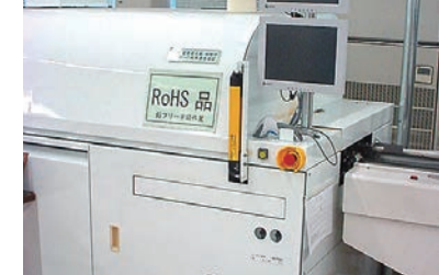
Renewed reflow furnace (Sagamihiro Factory)
