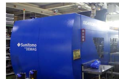
Renewal of energy-saving injection molding machines (Sagami-hara Factory)
