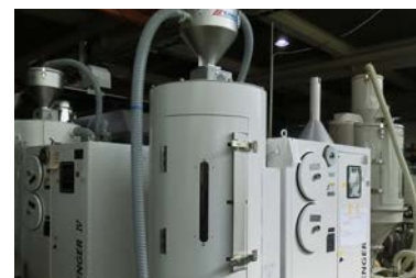
Replacing dehumidifiers with resin dehumidifiers consuming less electricity (Sagami-hara Factory)
