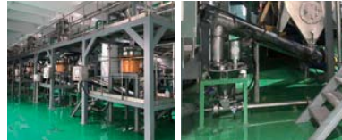
Continuous Transport System for low pressure and low density conveyance
