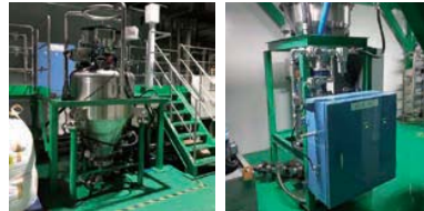
Continuous Transport Unit for high pressure and high density conveyance
