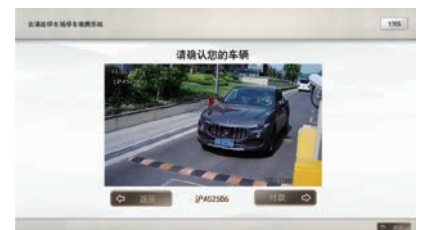
Vehicle confirmation screen An image of the vehicle taken at the entry is displayed. Proceed with the payment process if no errors are confirmed
