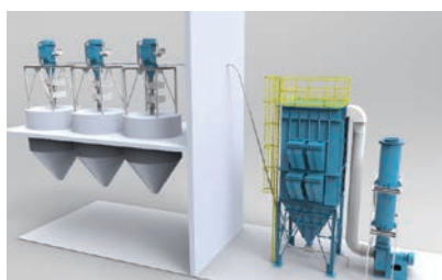
A figure in our proposal of modification of existing dust-collecting and pneumatic conveying system
