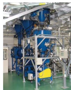
Pneumatic powder conveyance system test plant
